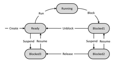
Assume a test always starts in the "Ready" state and ends when the system returns to the "Ready" state, so a test input consists of a sequence ("Ready", event, next state, ..., event, "Ready"), where all states except first and last one is different than "Ready".
